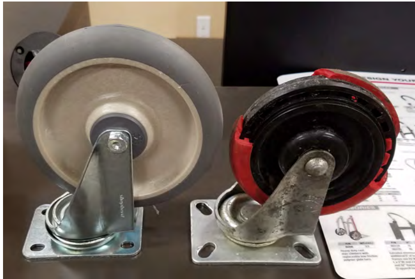
Solution: Replace broken wheel and increase to 6" Dia.
